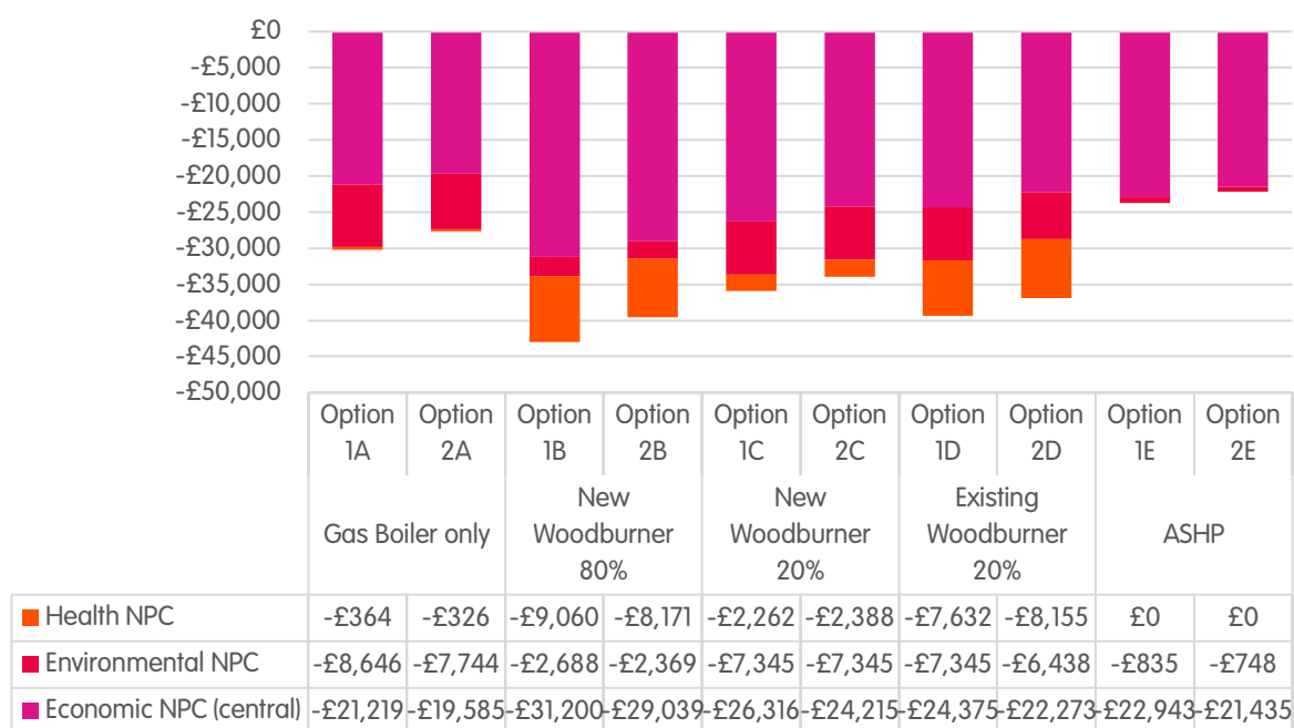
Figure 14 Combined economic, environmental and health costs across all scenarios over a 15-year lifespan
